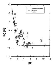
Fig. 6. Parks and Pohl uranium dioxide solubility data obtained under reducing conditions. Dashed line corresponds to UO2 solubility calculated under strict reducing conditions. Solid line is calculated with pe-pH pairs of values following the pairs corresponding to the equilibrium between U(IV) and U(VI).
