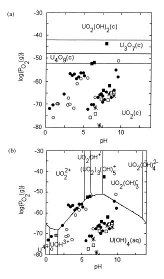
Fig. 2. Predominance diagrams of uranium as a function of logarithm of oxygen partial pressure and pH: (a) Predominant solid phases; (b) Predominant aqueous species. Experimental pe (corrected to log  $P_{02}$ )-pH measurements of the experiments: perchlorate (open dots), chloride (full dots), Cigar Lake (open squares), Jachymov (full squares), and Oklo (stars).
