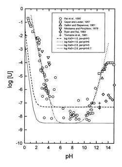
Fig. 5. Uranium dioxide solubility data obtained under nominally reducing conditions, corresponding to values extracted from the literature as given in the figure legend.
