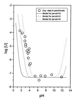
Fig. 1. Experimental solubilities as total uranium concentrations in solution for the dissolution of uranium dioxide in  $8 \times 10^{-3}$  mol dm<sup>-3</sup> sodium perchlorate test solution. Solid line corresponds to the calculated solubility.
