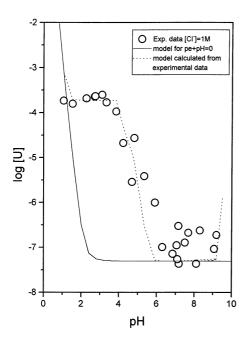
Fig. 3. Experimental solubilities as total uranium concentrations in solution for the dissolution of uranium dioxide in 1 mol dm-3 sodium chloride test solution. Solid line corresponds to the calculated solubility.
